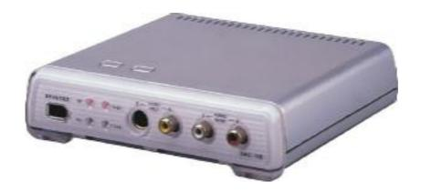
**Datavideo's DAC-100** bridges the gap between digital and analog video editing systems by providing instantaneous cross-format conversions. Using the DAC-100 to convert analog to DV let's you maintain the quality of your analog tape without generation loss.
